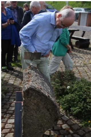
Calcium sinter in the Roman Canal
